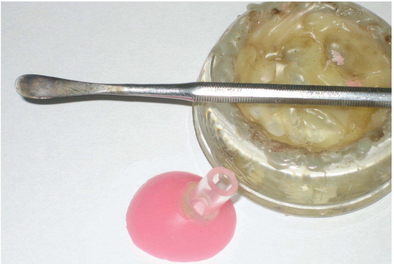
FIGURE 3: Sticky wax is used to secure tubing onto the wax shape.
